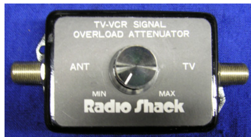
Figure 6.5: Attenuators reduce signal overload. They may be either variable (shown above) or fixed.
