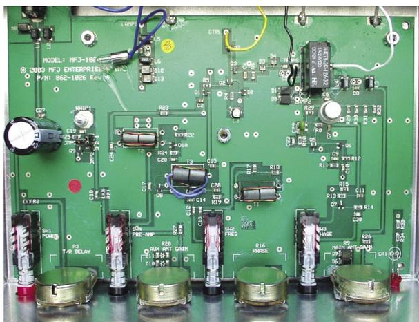
the “none” position, which was indicated as default in the manual, but with our “factory fresh” test sample, for some reason it was set at “moderate.” If you are using the whip antenna with the 1026, both stages are used and the jumper is set open (pins 1 and 2 on JMP2).
