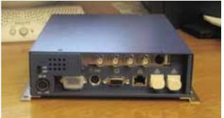
has 248 MB of RAM, a 30GB hard drive and built-in Ethernet, video, USB and serial ports. Windows XP Professional is provided as the operating system.
