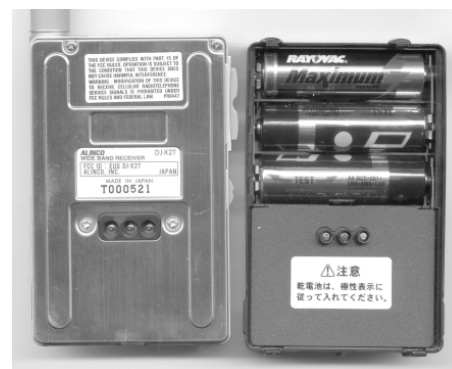
Figure 3. Rear view of DX-X2T (left) and the snap on, auxiliary battery pack/charger (right).
