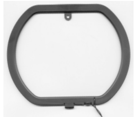
FIGURE 3. Supplied 7 inch AM loop antenna (base stand not shown).
