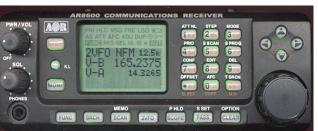
center frequency. Up to 50 frequencies may be skipped. The AR8600 will not stop on signals within 10 kHz of designated skip frequency.
