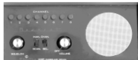
Figure 4. Early Electra Bearcat BC-L scanner. Note the lack of channel lockout switches.
