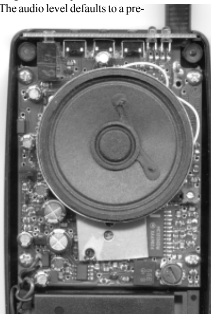
Figure 2. Tiger Scan uses surface mount components on a single board.
