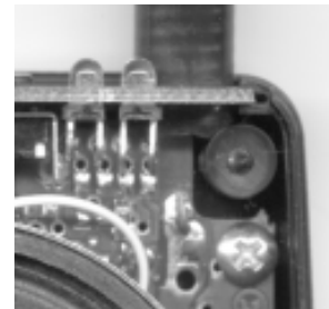
Figure 3. Permanent 2-1/2" helical antenna is glued to the top panel and soldered to the circuit board.
