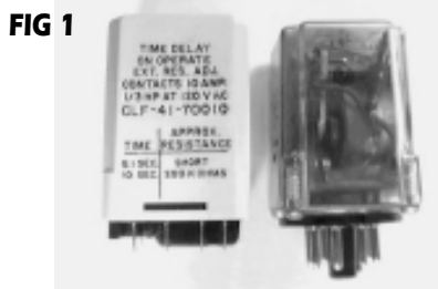
FIG 1 A handful of salvaged Potter & Brumfield plug-in relays were used to make a remote scanner controller.
