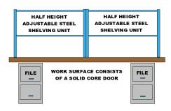
I cut the rails from a full height shelving unit in half to yield two half height shelving units. They rest atop a solid core door, again supported by a pair of filing cabinets.
