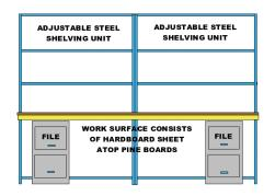
home made radio desk consists of two shallow 2-drawer file cabinets supporting a pair of 2 by 10 planks fastened side by side. A layer of 1/4 inch hard board nailed to the top provides a hard work surface for writing. Two coats of Krylon clear lacquer spray seal the hard board against moisture. Strips of 3/4 inch molding (not shown) guard the edges on 3 sides of the desk top, although the molding isn't essential.
