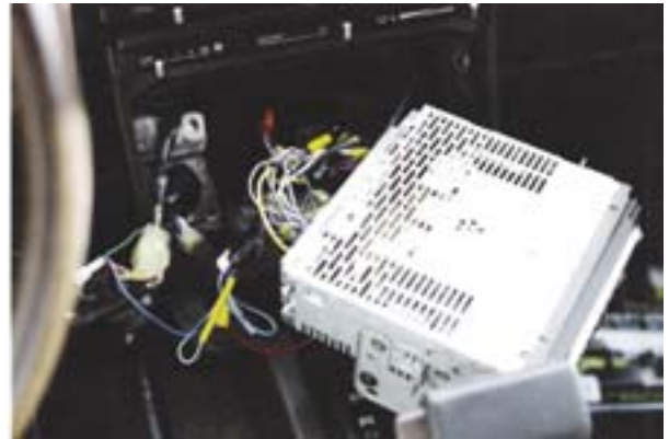
Use small wire nuts to connect the new wiring harness to your stock speaker and power wires. Installing the radio requires patience and a couple of hours of your weekend. (Courtesy: Author)
