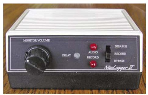
are inserted into the scanner and tape recorder, the wall adaptor is plugged in, and the monitor volume is adjusted for comfort while a signal (like your local weather channel) is being received. A small screwdriver (not included) is used to adjust the front-panel input level as revealed by an illuminated LED; a second LED reports the activation of the tape recorder. That's it.
