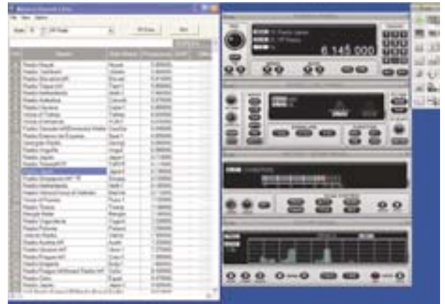
Figure 2 - 1500 shown in the component format in the center. The "Tool" Bar is at right and the memory channel editor (log) at left
