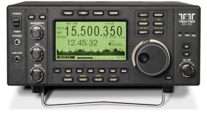
While the bar graph S-meter is calibrated for the conventional 50 microvolt signal equaling S-9, the entire meter is compressed into a one-inch space, with each 1/8-inch reticle division representing nearly 4 S-units (20-24 dB) of signal level change. While an adjacent numeric readout in 1/8-inch characters is provided, it is distracting to have to refer constantly to a changing number to get a fix on relative signal strengths. But it does provide reference levels.
