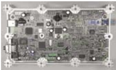
The G303e Control Board
