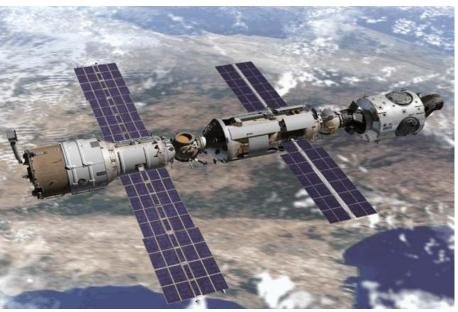
Figure 7 ISS Early Stack (Zarya (left) Zvezda (middle) docking port (right)
