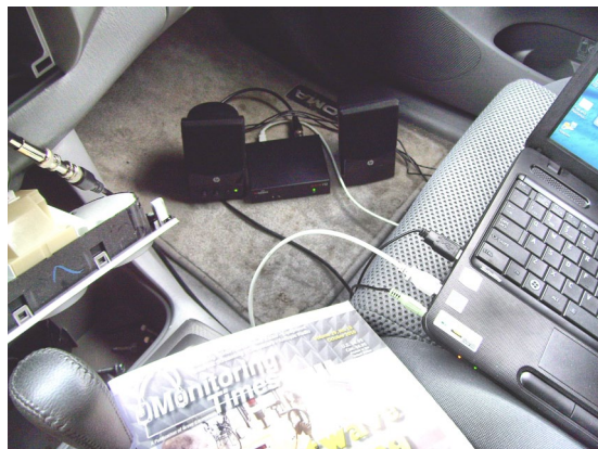
Photo 1. SDR-IQ and USB-powered speakers on the floor are connected to the laptop, with the center radio and environmental controls removed to gain access to the radio antenna.
