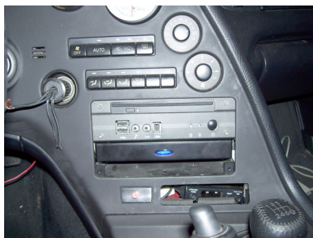
Photo 4a (above) shows the in-dash PC mounted in the space formerly occupied by the AM/FM/CD player. The pop-out monitor is directly below the PC. Photo 4b (below) shows the monitor in its extended position, with Microsoft Windows XP on the display.
