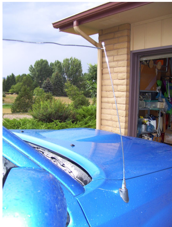
Photo 2. Replacement aluminum antenna mounted on truck with insulated wire running diagonally across the roof and into the bed of the pickup on the opposite side. The antenna bows slightly in order to make the wire as tight as possible.
