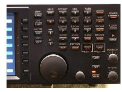
While the receiver does not have trunk tracking capability, it does provide APCO P-25 digital voice decoding, the fastest growing digital voice technology to be encountered on public safety frequencies in the VHF/UHF spectrum.
