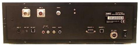
an I/Q out, DB-9 and modular digital control connectors, and a multipurpose port which provides two 12 VDC @ 50 mA lines for antenna switching, and an AGC control line.
