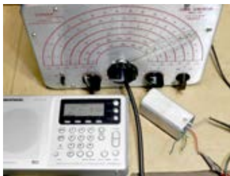
A Conar 280 signal generator is tuned to exactly 455 kHz as indicated by zero beating its second harmonic at 910 kHz on a Grundig YB-400PE digitally-tuned radio.
