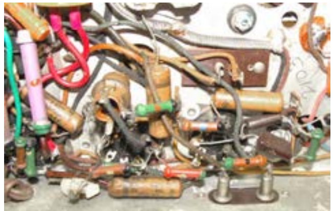
To be this compact, the EC-1's wiring had to have been installed in layers. Author's Photo.
