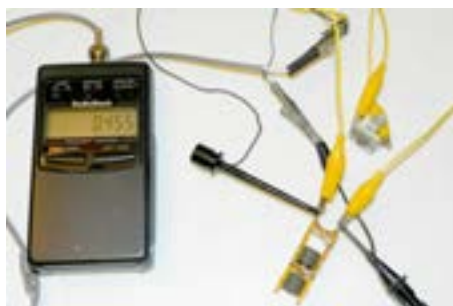
Testing an IF transformer winding to determine capacitance needed at 455 kHz resonance by adjusting a trimmer capacitor on clip leads. With the ferrite slug at its center, the needed cap measured 180 pF. With the slug at its extremes, the needed cap ranged between 160 and 202 pF.
