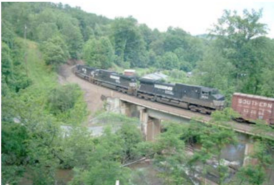
Three large modern Norfolk Southern diesel locomotives are working hard to get a relatively short freight train of only about 50 cars up the major grade on the NS "S" line between Old Fort and Asheville, N.C. This view is from a backcountry road near the community of Graphite. In flat country, those same three engines would be able to move a train of up to 150 freight cars. This section of the S line is known as "The Loops" because the tracks twist back and forth through several valleys to gain altitude.
