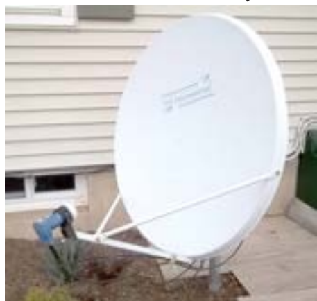
Photo 1. Author's Ku band dish aimed at Galaxy 19 (97W) , the mother lode of FTA radio fare.
