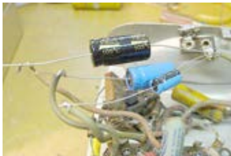
Temporary installation of electrolytics allowed room for possible additional diagnosis and component replacement.
