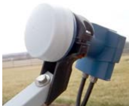
Photo 2. Two-port LNB; one coax goes to my TV, the other goes to the FTA "radio."
