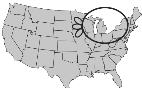
From southeastern Minnesota, a typical beam antenna aimed at New York puts most of the rest of the country off the side or back of the pattern, reducing signal strength or forcing frequent re-aiming. See text.
