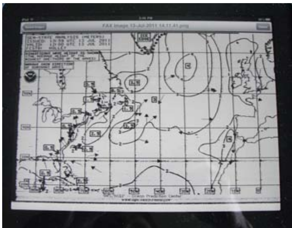
NOAA WEFAX showing Sea State Analysis received on an iPad via Black Cat Systems HF FAX App.
