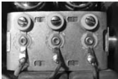
The (left to right) oscillator, r.f. and antenna trimmers sit atop the tuning capacitor frame.
