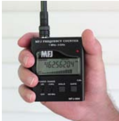
The MFJ-886 in action, showing the 10 digit frequency display and the LCD bargraph at full deflection.
