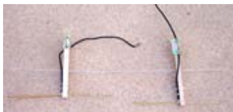
50 Ohm on the left, 75 Ohm on the right base copper wire, and brass/copper hobby tubing have all been used.
