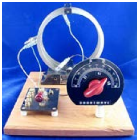
My Second Shortwave Crystal Set As Originally Built.
