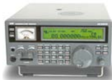
AOR AR5001D ($4,500) top-grade, wideband receiver takes you anywhere in the spectrum you'd like to go from 40 kHz to 4150 MHz. (Courtesy: AOR U.S.A.)
