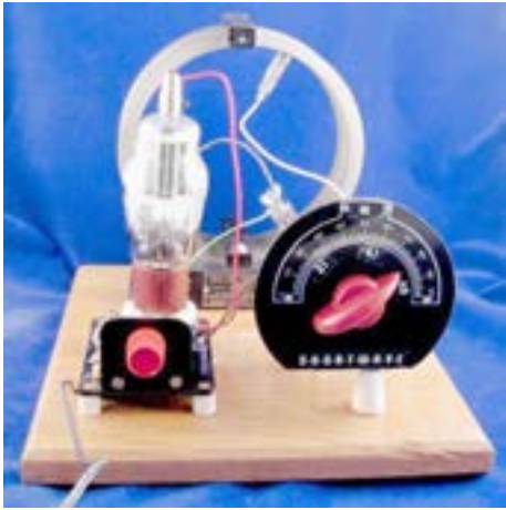
Rebuilt second shortwave crystal radio, now a tube radio.
