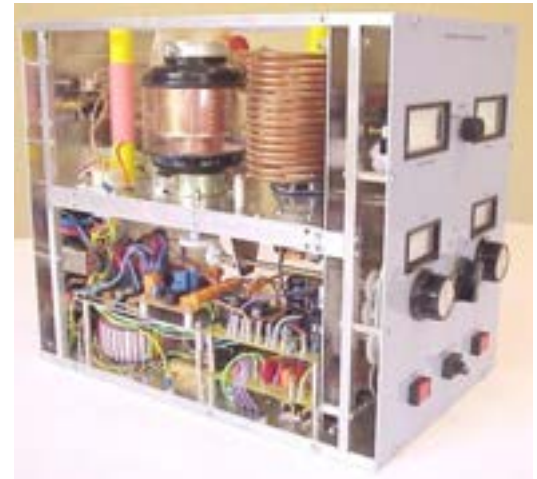
RF power amplifiers can be a "rite of passage" for advanced home-brewers, and some, like this 160-10m "desktop kilowatt," designed, built and tested by Mark Marsden, G4AXX, over a four-year period, are real works of art. Built around an Eimac 4CX1000A triode, the amp runs on 230 VAC and puts out 1400 W PEP from 25 or 100 W of drive (selectable). See more at www.granta.g4axx.com/linear.php3 . (Courtesy: Mark Marsden G4AXX.)
