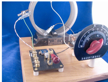
Shortwave crystal set close-up shows galena crystal detector.
