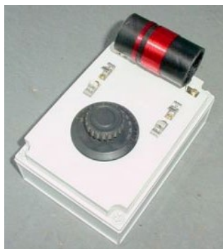
A Simple Shortwave Crystal Radio.
