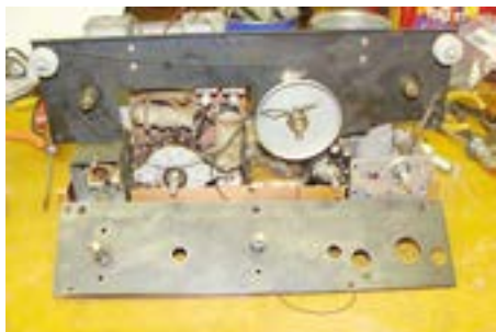
With the lower mounting plate out of the way, I could now service the dial cords.
