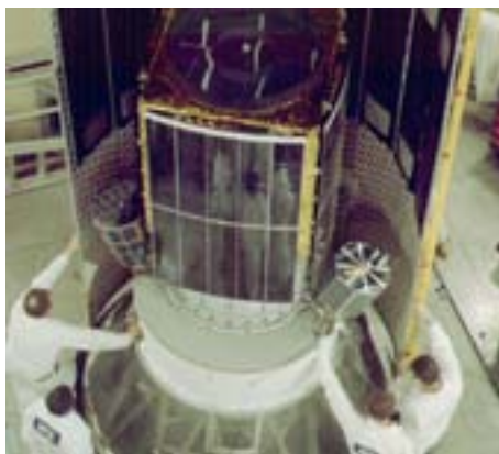
AO-7 is shown here mated to the upper stage of its Delta rocket. AO-7 is shown at the bottom right, next to the much larger main payload. (Courtesy: AMSAT)
