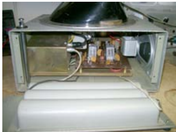
Figure 2. RDF 304 with rear panel removed. “D” cell battery tray is shown in foreground, facing down on the bench. Luckily, it shows no signs of corrosion. (Photo by Kevin Carey)
