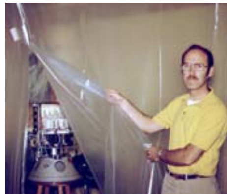
AO-7's final assembly "Clean Room" consisted of stud lumber and plastic sheeting installed in the basement of Dick Daniel's (W4PUG) home in suburban Washington, DC. Despite such sparse assembly arrangements, AMSAT has never had a satellite rejected by a launch agency because of contamination. (Courtesy: AMSAT)
