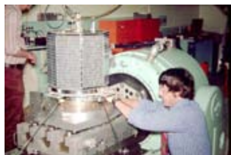
Jan King, W3GEY, prepares the AO-7 satellite for vibration testing. (Courtesy: AMSAT)
