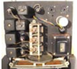
Fig. 4. Our chassis matches the layout of the Meissner broadcast and shortwave Receiver (Fig. 2) rather than that of the broadcast only set (Fig. 1), but it is definitely the broadcast model (see text).
