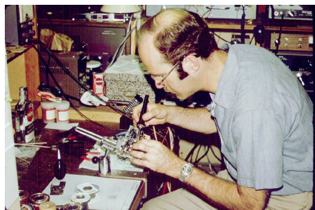
AMSAT's satellites are often built in the basements and garages of its experimenters. Here Dick Daniels, W4PUG, solders components into one of AO-7's electronic modules. (Courtesy: AMSAT)
