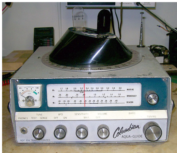
Figure 1. The Columbian Aqua-Guide is a solid state radio direction finder covering longwave, AM broadcast, and MF marine bands. I’m starting it up for the first time in this column. (Photo by Kevin Carey)
