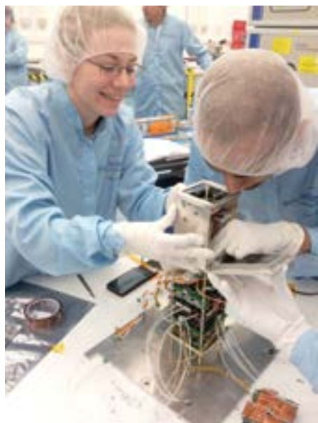
STRaND-1 took just 3 months to build and uses a Google Nexus One smartphone with an Android operating system. (Courtesy: AMSAT-UK)
