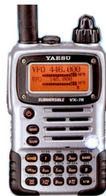
Yaesu VX-7R ($370): A Technician Class four band HT that transmits on 6 meters, 2 meters, 440 and 220 MHz FM and receives broadcast band AM and FM, Air Band and shortwave from 1.800 - 30 MHz. (Courtesy: Universal Radio)
