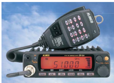
Alinco DR-06T ($272) compact 6 meter FM portable rig works at home or in the car. Work FM repeaters or simplex FM with three power settings. (Courtesy: Universal Radio)
