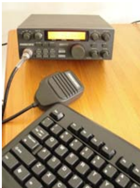
Uniden 2510 and its twin, the Radio Shack HTX-10, were great 10 meter rigs: 25 watts output, all-mode, compact, solidly built and still selling for about $100 used. I paid $150 for mine new more than 20 years ago and worked the world from the front seat of the car. (Courtesy: Author)
