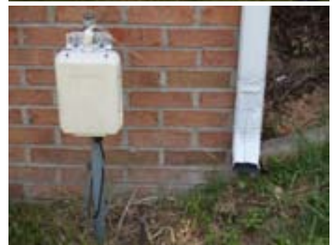
In 2010, during a year of casual operating and rather poor overall propagation, Bill Mabry N4QA, of Radford, Virginia, made 560 contacts on 160 through 6 meters, 558 of which were at 5 W or less, using this downspout as his antenna! Fed with an ICOM AH-4 auto-coupler for lightning-fast band changes, Bill calls the antenna GADS, short for Gutter and Down Spout. In addition to working QRPDX on four continents, Bill worked all states except Hawaii and most Canadian provinces. If Cycle 24 perks up in 2011, look for Bill to be busting pileups in every direction! (Photos courtesy: N4QA)
