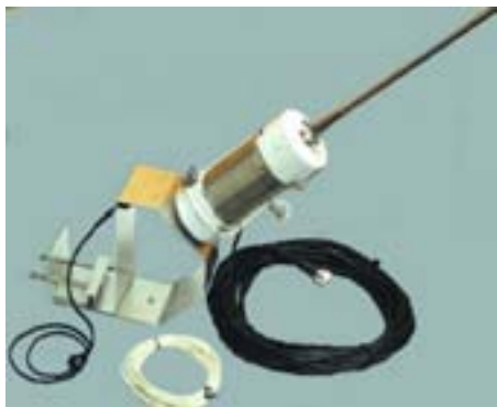
MFJ's nifty "apartment antenna" gets even high-rise dwellers on the air with a minimum of fuss. (Photo courtesy MFJ Enterprises)
