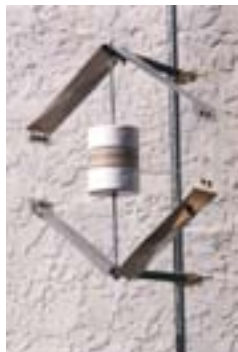
A clever and effective solution for getting wire antennas up in the trees. (Photo courtesy E-Z Hang)
