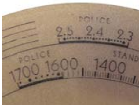
Segment of Philco tuning dial shows both police bands.
