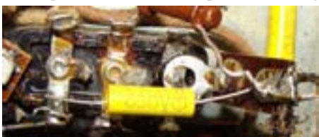
External coupling capacitor bypasses internal block unit. Added tie point is at right (see text).
