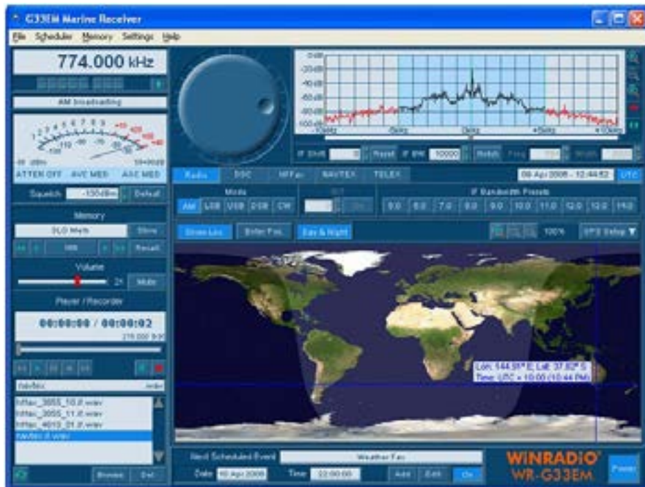
Figure 2: The upper-right screen displays the signal contents with adjustable bandwidth and notch filter. The zoomable world map shows the area of Earth currently illuminated by the Sun.
