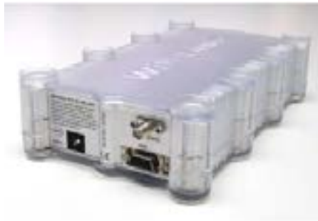
Figure 1: The rugged case of the WiNRADiO G33EM has three ports for 12 VDC power, antenna, and USB interconnect.
