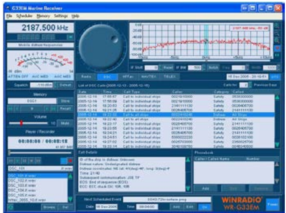
Figure 3: Digital selective calling (DSC) logs and records distress messages for later playback or printout
