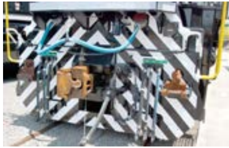
The event also provided an opportunity to get a close-up look at the new locomotives. Here, the rear of one of these new units has the EP (electro-pneumatic) braking equipment mounted just to the right of the coupler.
