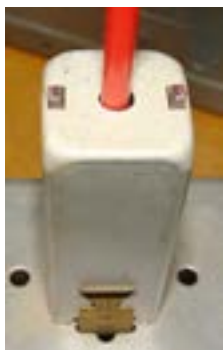
Attempting an IF adjustment using a non metallic tool.
