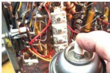
A couple of sprays with contact cleaner smoothed out the bandswitch operation.
