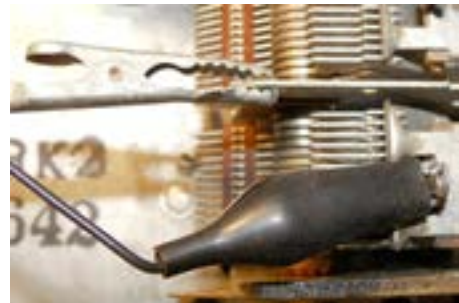
For IF alignment, the signal generator is connected between the antenna capacitor stator and ground.
