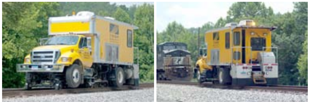
Front and rear views of Sperry Rail Services truck 983 at Huddleston, Va. The scanning equipment for detecting rail flaws is between the two highway tires. These trucks are set up so that they can operate in reverse while on the rails.
