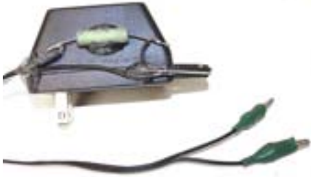
The “wall wart” handy dandy transformer tester. It’s definitely not pretty, but it does the job!
