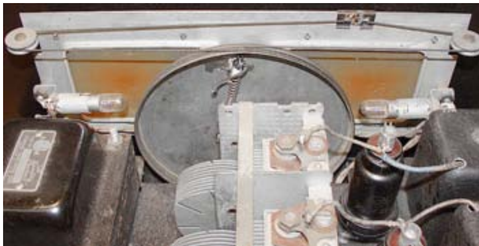
The Meissner’s sticking dial drive resisted all correction attempts, then got fixed by luck (see text).
