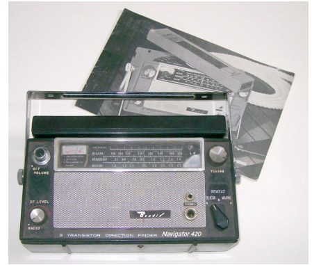
Our next LF restoration project: a Bendix Navigator 420 RDF receiver
