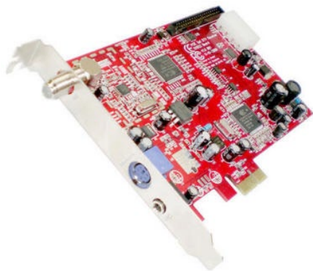
DVB-S2 PCI3 Free-to-Air PCI-based FTA satellite TV receiver card ($100). (Courtesy: Sadoun.com)
