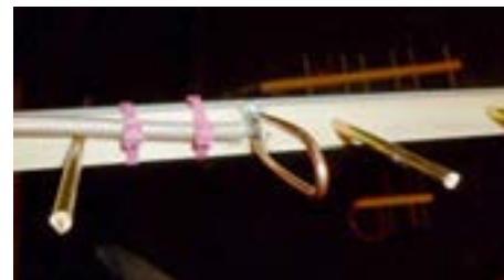
Photo 4: How to attach the coax.
