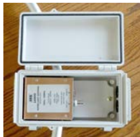
AOR LA800 Active Antenna ABS Plastic Box with Top Element Circuitry
