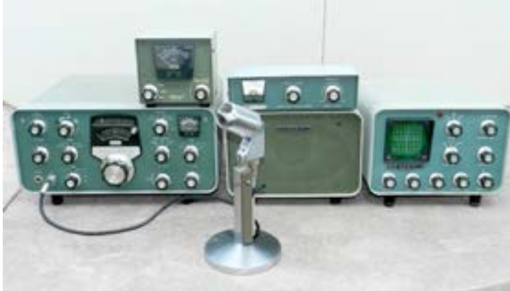
Complete Heathkit SB101 station. Left to right bottom: SB-101 transceiver, SB-600 speaker (with HP-23B power supply inside) and SB-610 Signal Monitor. On top from left HM-102 RF power meter and HM-15 SWR meter. The official name of the HM-15 as printed on the front panel is "reflected power meter" but most hams simply call it an SWR meter. Foreground HDP-21A mike.
