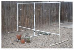
Above is my simple antenna used to detect TV channel 3's video carrier.
