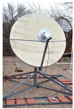
The dish mounting hardware was designed for a fixed elevation and needs modifications. I plan to modify the mount to allow it to move in elevation only. In this mode, the dish will scan the sky with the earth's drift or rotation. I purchased a new cylindrical feed-horn from Radio Astronomy Supplies that is designed to operate on 1420 MHz.
