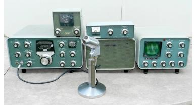
Complete Heathkit SB101 station. Left to right bottom: SB-101 transceiver, SB-600 speaker (with HP-23B power supply inside) and SB-610 Signal Monitor. On top from left HM-102 RF power meter and HM-15 SWR meter. The official name of the HM-15 as printed on the front panel is "reflected power meter" but most hams simply call it an SWR meter. Foreground HDP-21A mike.
