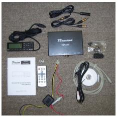
The above photo shows the Directed Electronics solution. It's simple enough: 12V power (switched and unswitched), PC/front panel interface, stereo line out jacks, antenna in and antenna out RF jacks. Since the interface jack is meant to be attached to the included front panel, a separate cable, available from Mo-Co-So (MCS-MJS-HDR), is needed to connect the box to a USB port. The cable also works with the Visteon HDZ-300. Below shows how to connect this device to a PC.
