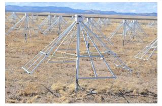
Note that the antenna elements are somewhat aligned with an east-west and north-south orientation. The antennas are not in perfect lines due to phasing of the pattern requirements. There is a coax cable run from each antenna into a small building. Each cable is lightning protected.
