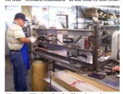
Photo A- Winders for the fiberglass whips
