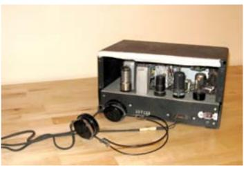
Hallicrafters S-38B radio showing tubes and original Trimm headset.
