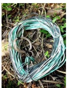
This is my camping antenna. It's made from 240 feet of 12-gauge insulated wire. It's pretty heavy. If you were hiking some distance, you'd probably want to go with lighter bare-copper wire.
