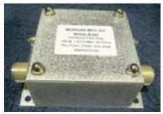
Figure 3. A Morgan Manufacturing bandpass filter
