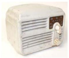
The Arvin Model 444A as found. The knobs may not be correct for this model, though they appear to be Arvin.
