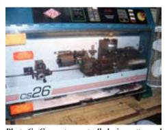
Photo C - Computer controlled wire cutter and stripper
