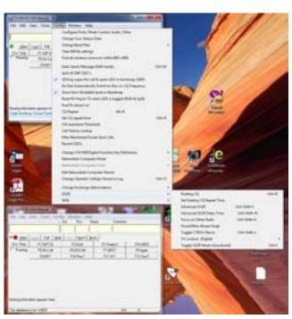
Figure 5. N1MM software creates two windows, one for each radio (or for two VFOs in the case of SO2V). Here, the Config menu has been selected to show the SO2R entry, which brings up another window to allow you to select relevant parameters for SO2R.
