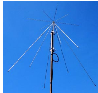
AOR DA3000 ($120) wideband discone antenna covers from 25 to 2,000 MHz. (Courtesy: AOR)
