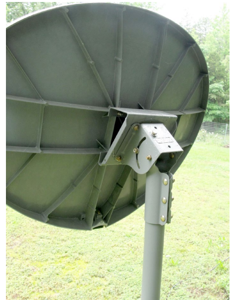
Back of the Channel Master dish shows heavy-duty mount. (Courtesy: Author)
