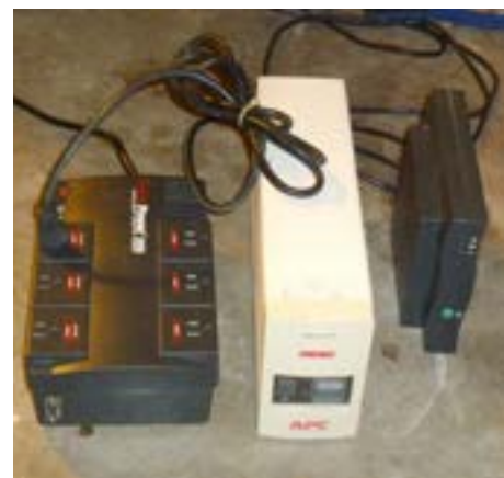
Photo B Daisy Chained UPS
