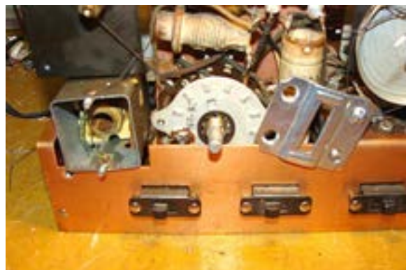
Odd piece of hardware from junk box was used to support drive pulley temporarily in working position (see text).
