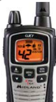
Midland GXT860 five watt GMRS HT; buy the boom/mic headset and hold the HT away from your body when transmitting . (Courtesy: Midland Radio)
