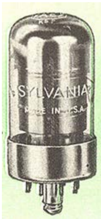
Photo of Loktal tube shows groove in keyed locating post.
