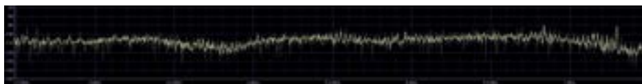
This WiNRADiO G39DDC spectrum scan from 3.5 to 7.5 MHz shows the “lumpy and bumpy” nature of the composite RF background noise typically experienced by hams and SWLs in urban and suburban environments. (Scan courtesy of Bob Grove W8JHD)
