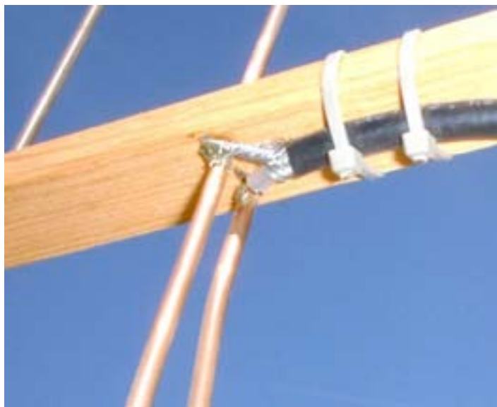
Photo F - Close up of the coax attachment
