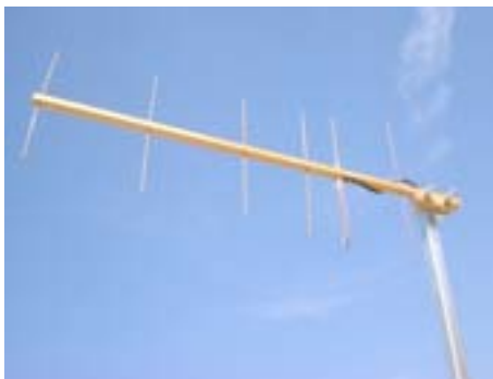
Photo E - 460 MHz Beam antenna
