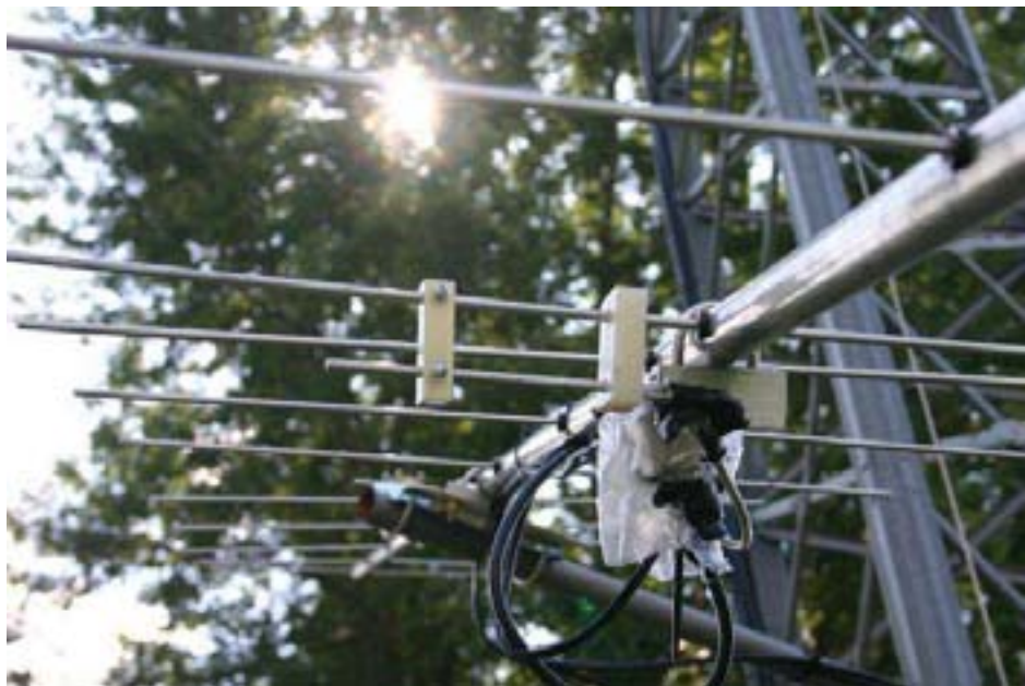
Author’s home-brew FltSatCom antenna showing the gamma match. (Courtesy Bob DeVarney W1ICW)
