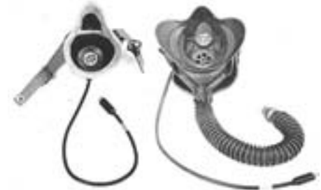
Fig. 4. At left, a carbon mic unit is installed in a noise reducing shield that was strapped over the user's nose and mouth. The same effect could be obtained (at right) by building the mic into an aviator's oxygen mask.
