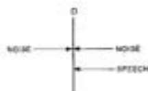
Fig. 7. In the lip mic, noise impinges equally on both sides of pickup diaphragm "D," thereby canceling itself out. However, speech sounds fall mainly on one side of the diaphragm and are transmitted.
