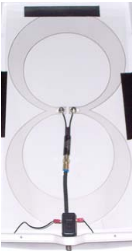
Photo A - Printed Ink TV Antenna
