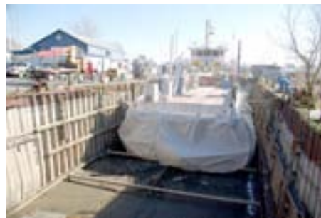
The ferry Quinte Loyalist undergoing 5 year inspection and refit before winter operations. Vessel operates all winter utilizing a bubble system to keep the channel free of ice.
