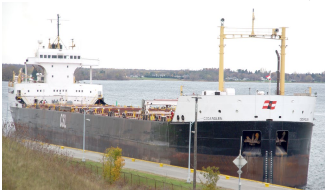
Cedarglen approaching Iroquois lock. This ship utilized the stern of an ocean vessel and a new Great Lakes forebody which was attached. This was one ship I particularly wanted to photograph as a similar ship went to scrap this year.
