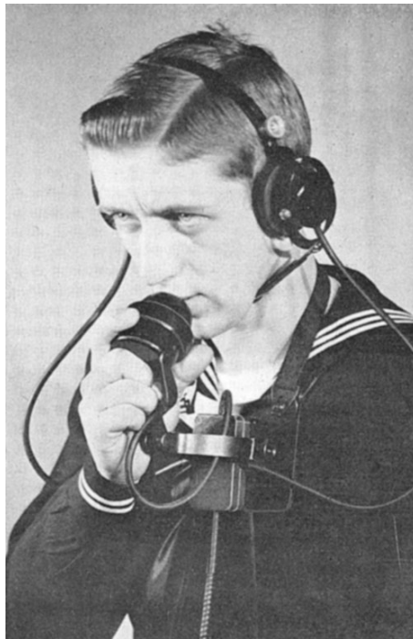
Fig. 8. In marine applications, sound powered phones replaced speaking tubes for emergency communications. In military applications, the phones replaced battery powered units in Arctic and tropical climates (see text).
