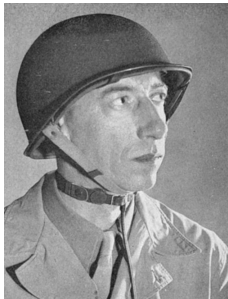
Fig. 5. Here, reduction of external noise is accomplished by fastening two carbon mic units to a strap fastened tightly high on the user's neck. Reproduction of this throat mic was less than perfect, lacking high frequencies.
