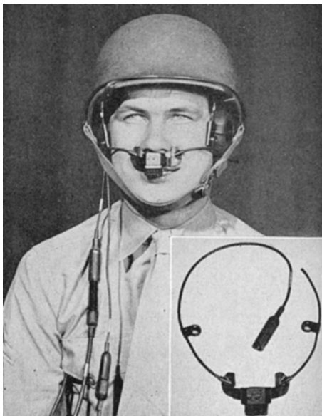
Fig. 6. The odd looking lip mic reproduced a wider frequency range than the throat mic, and used a simple, but ingenious design for minimizing noise pickup (see Fig. 7).
