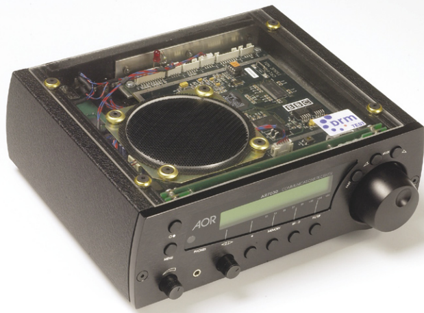
Dawn of the shortwave digital age. This AOR 7030 SW radio has been retrofitted with the necessary hardware to allow it to receive DRM broadcasts. (Courtesy: BBC R&D)
