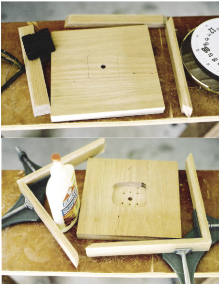
The three piece desk clock in furniture clamps. These clamps are overkill, you can use much smaller (and cheaper) clamps for a project this small. Rout a space on the back of the dial board on the 24 hour clock to insert the special quartz 24 hour movement. (Courtesy Author)
