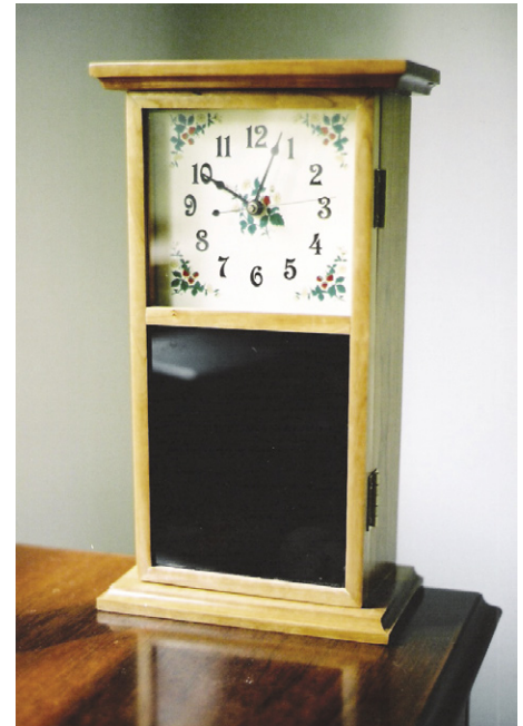
Case for the Shaker style atomic clock is just 5 pieces glued together. Facing edges of the top and bottom are routed for a traditional look. (Courtesy Author)
