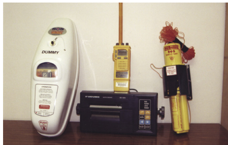
Simulated radio equipment for radio course. Clockwise L to R Dummy EPIRB, Waterproof VHF portable for survival craft, SART, Navtex receiver
