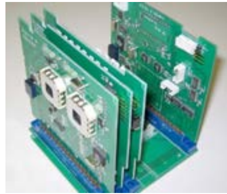
The SEEDS-2 satellite features side mounted, plug-in circuit boards (Courtesy: Nihon University)
