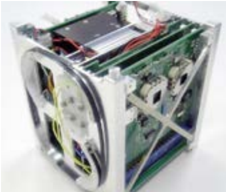
The SEEDS-2 satellite features a unique "truss" structure and a plastic form to secure its coiled 70cm downlink antenna for launch. (Courtesy: Nihon University)
