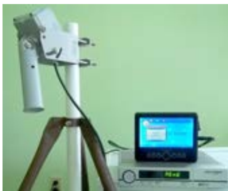
Bench-testing dish mover.
