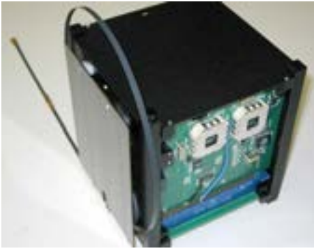
The SEEDS-2 satellite with top and bottom covers attached. (Courtesy: Nihon University)
