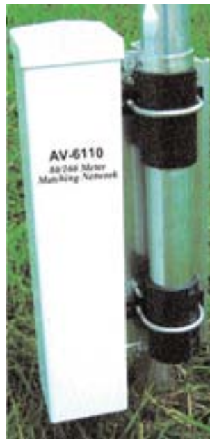
HyGain's AV-6110, a matching network that makes a 43 foot vertical actually WORK on 160 and 80 meters. (Photo courtesy MFJ Enterprises)
