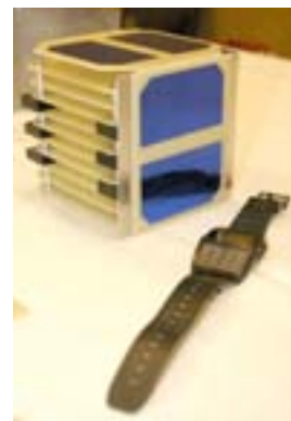
A full-scale structural engineering mockup of the Fox-1 satellite showing its multiple internal circuit board locations. Note the wristwatch used for size comparison. (KB1SF Photo)
