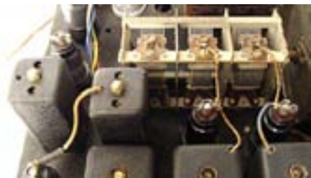
The main three-section tuning capacitor with its three trimmers is at the top of the picture. Just below it and to the left are the two i.f. transformer cans. At the bottom are the three "Universal Replacement" coils (see text).
