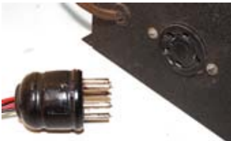
Before starting this month’s session, I made up a speaker plug to fit the socket at the back of the set.
