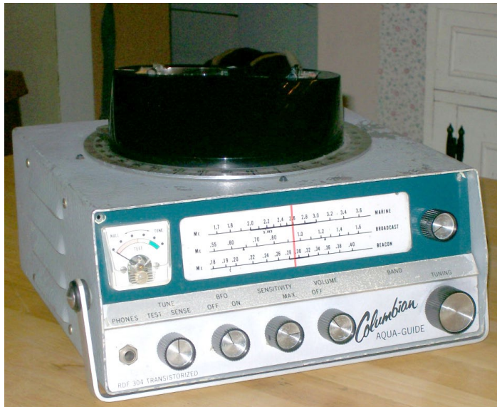
The completed RDF-304 project. The radio should now provide years of service on its Longwave and two mediumwave bands.
