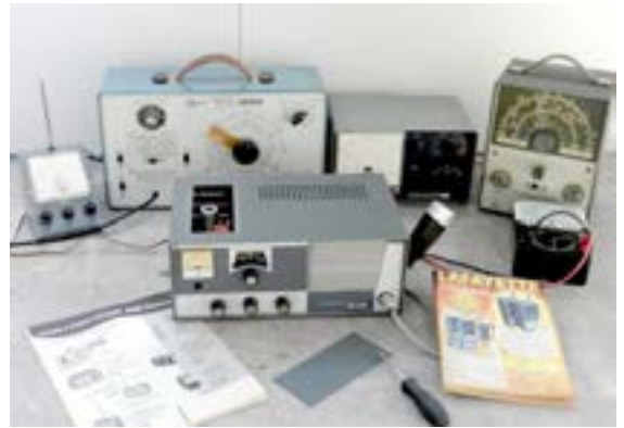
An all-Lafayette test-bench: Equipment from left: TM-16A field strength meter; LC-4 Capacitor-resistor checker; Model 174 VTVM; KT-208 signal generator and tracer; 30,000 ohm/volt VOM model 99-5004.
