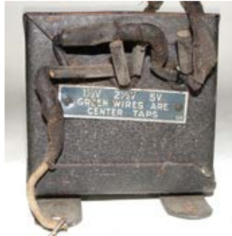
Power transformer removed from junked 1929 era radio. Note the three different heater voltages.
