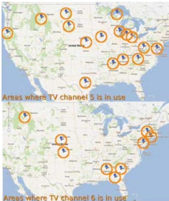
TV channels 5 and 6 are off-limits for an "FM expanded band" in heavily-populated parts of the country. (Courtesy: Doug Smith & Google Maps)
