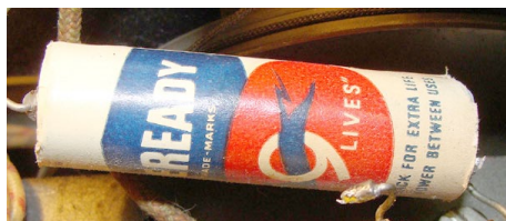
Ancient Eveready penlight cell had been soldered in to replace a dried-out Mallory bias cell. As it still provided 1.5 volts on the nose, I left it in place.
