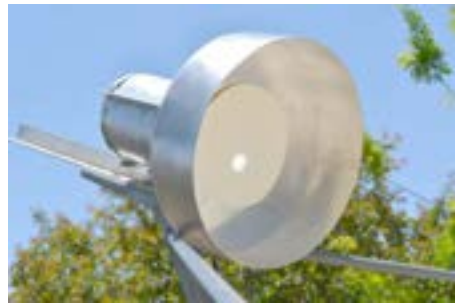
Reflected image of the sun by mirror almost centered.
