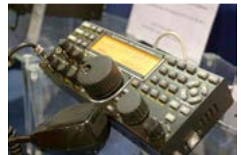
The Elecraft K3/0 Mini is a slim-line faceplate that, when used with the RemoteRig 1258 MkII's, can completely control your K3 remotely.
