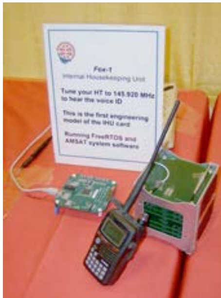
The engineering model of FOX-1A's Internal Housekeeping Unit (IHU) was broadcasting greetings on 2m at the 2013 Dayton Hamvention®. (Courtesy: Author)
