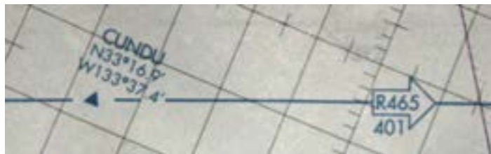
Portion of North Pacific Route Planning Chart showing waypoint CUNDU on track R465.
