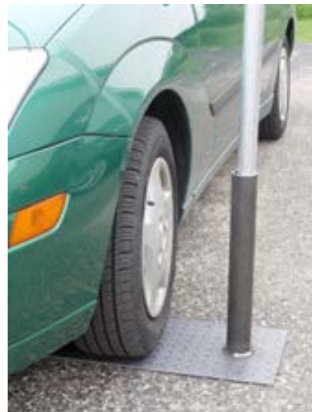
This “quick and dirty” drive-on mast mount isn’t backpack friendly, but it’s foolproof and amazingly rigid. (NTOZ Photo)
