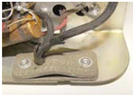
Rivets on the unusual cord restraint had to be drilled out so it could be removed (see text).
