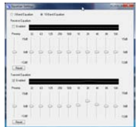
Many modern DSP-based rigs include some type of RX and TX equalization. Shown here is the RX/TX equalizer built into the FLEX-1500 SDR, which offers up to 10 EQ bands and +15/-12 dB control range. – NT0Z
