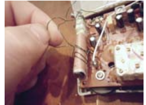
You can hook up an external antenna to your AM radio by simply wrapping a few turns of enamel-coated magnet wire around the internal ferrite antenna. Connect one end of this wire to your antenna and the other to ground.
