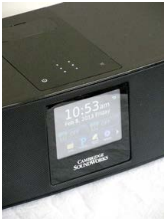
Top-mounted, lighted, touch-sensitive on/off switch, mute and sliding volume controls, all flush with the cabinet's surface. Note access door for iPhone/iPod docking.
