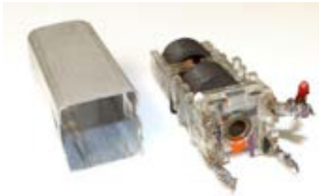
Fig. 2. The transformer cover slides right off after unbending two metal tabs.. Note threaded powdered-iron adjustment cylinders and brass rivet (see text).
