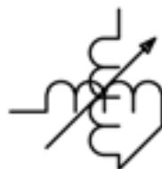
Fig 4 Variocoupler schematic symbol
