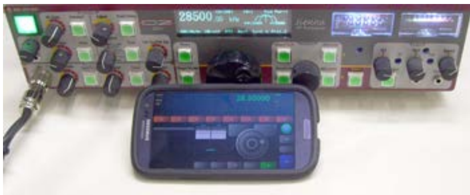
Sienna with Pocket Transceiver app running on a Samsung Galaxy SIII. The "cell phone" is connected to HRD's server via Wi-Fi. The HRD server is running on a PC that is connected to the rig (in this case a DZKit Sienna) via an RS-232 port.
