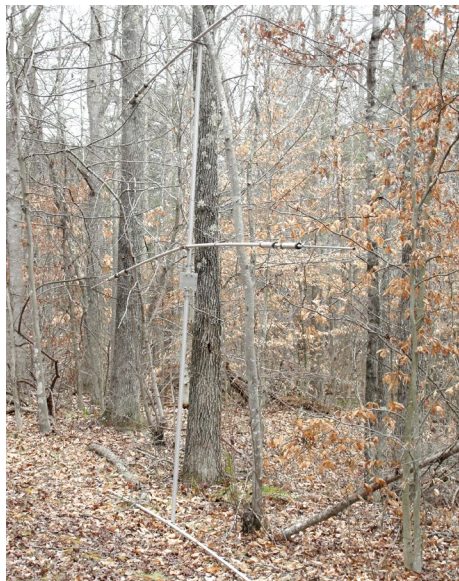
Tree supported three element HF beam provides Xtreme operating action.
