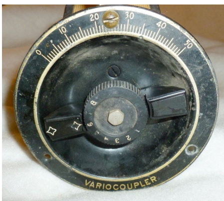
Photo 3 Variocoupler with position and switch controls
